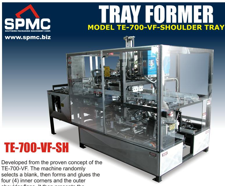
shoulder flaps. It then presents the finished tray to the operator for handloading of the product or is discharged onto the customer's take-away conveyor.
