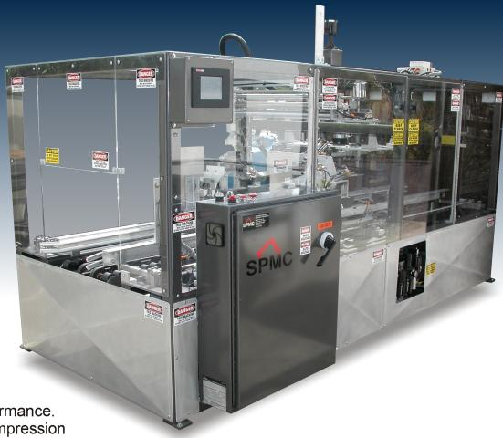
A durable, fully automatic machine engineered for round-the-clock performance. Positive top and side compression produces a sealed container, which offers superior product protection. This machine has a straight forward operation with simplified pneumatic functions, providing reliability and easy maintenance.
